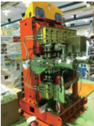
Fig. 4. New in-vacuum undulator for BL4U STXM beamline.
