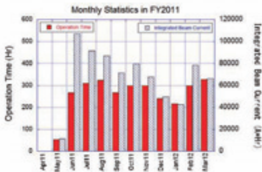
Fig. 1. Monthly statistics in FY2011 (upper) for the operation time (red bars) and integrated beam current (blue dashed bars).
